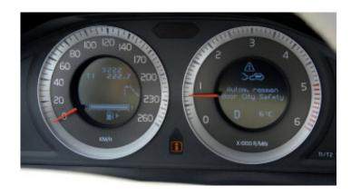
"City Safety" only works when the driver doesn't actively participate. In other words: the speed should be constant. After braking automatically, the car will be stopped for one full second. After that the computer releases the brakes. Those who didn't recover from the initial scare, will hit the car in front after all. Finally, the laser only works on reflective surfaces; therefore the XC60 doesn't brake for bicycles or pedestrians.
