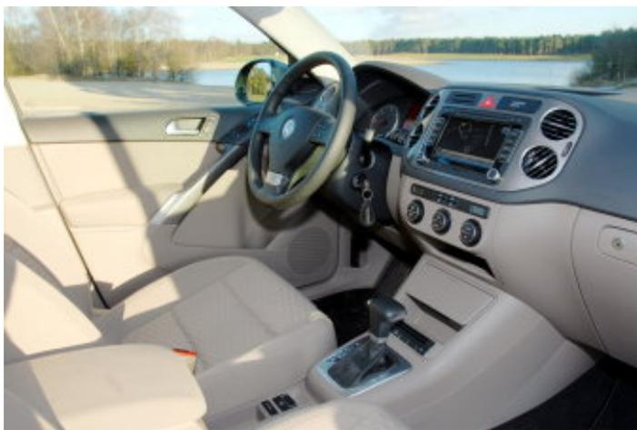
The most important of which is the combined audio, mobile and navigation system (&rdquo;RNS 510&rdquo;). It brings together all the contemporary technology (Bluetooth, MP3, audio from SD-cards, an internal hard drive, etc.), has pleasingly clear graphics and is easy to use. This system can be upgraded to use with a reversing camera thus making parking very easy (a must have!). Adaptive headlights and an electric parking brake are all part of the equipment.
