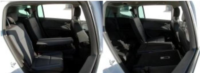
As of now the back seat consists of three separate seats. They are fitted on rails, so they can be moved to create either more legroom or more space for luggage.
