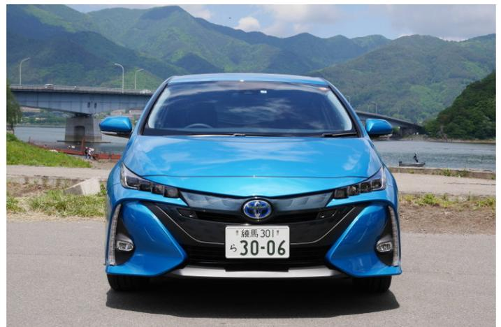
Toyota did realise that an "intermediate" vehicle was a possibility! The Prius ("forerunner") combines an electric motor and a petrol engine in one vehicle. Clever mechanics ensure smooth transition from one power-train to the other. Also, both engines can combine their power for maximum performance, if so required. The result is a quick, comfortable car that uses roughly half the fuel of a conventional car of the same caliber.
