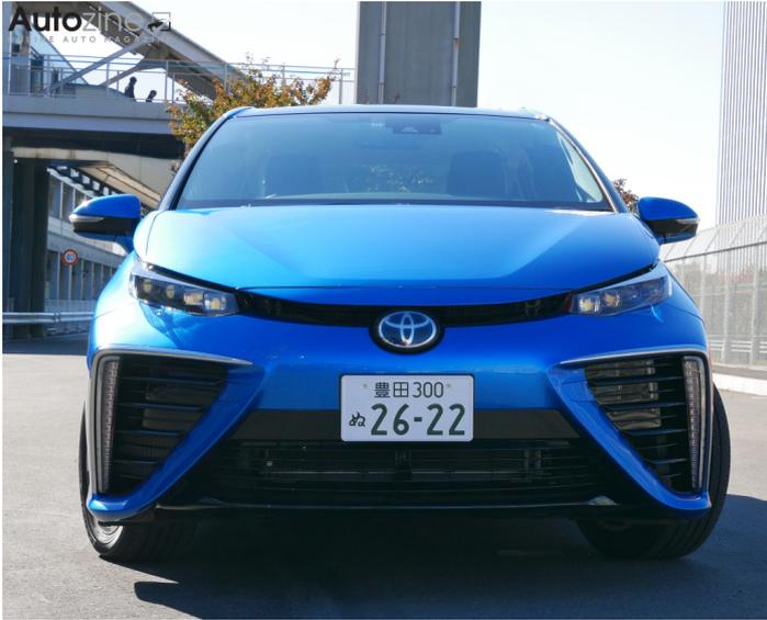
The Toyota Mirai is propelled by an electric motor, just like an electric car. The difference is that the required electricity is not only supplied by a battery, but mainly by a small on-board "power plant". The so-called "fuel cell" converts hydrogen, which is stored in gaseous form in a tank, into electricity and water. The water that the Mirai emits is so pure, that one could (theoretically) drink it.
