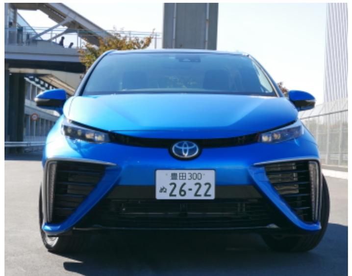
The Toyota Mirai is propelled by an electric motor, just like an electric car. The difference is that the required electricity is not only supplied by a battery, but mainly by a small on-board "power plant". The so-called "fuel cell" converts hydrogen, which is stored in gaseous
