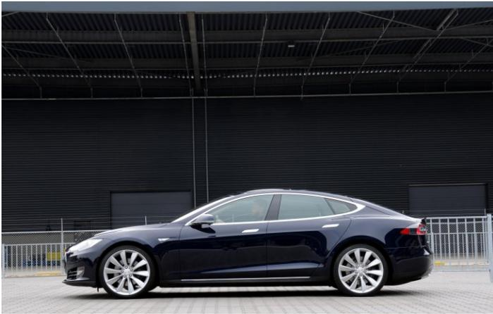
In real life the Model S can cover about 400 km (250 miles) on a full charge. After that there's no emergency engine to fall back on. This range is significantly better than that of other electric cars, yet painfully small compared to conventional mile munchers. And there's the big problem: cars like these are bought primarily to cover huge distances, and 400 km isn't exactly a long journey.
