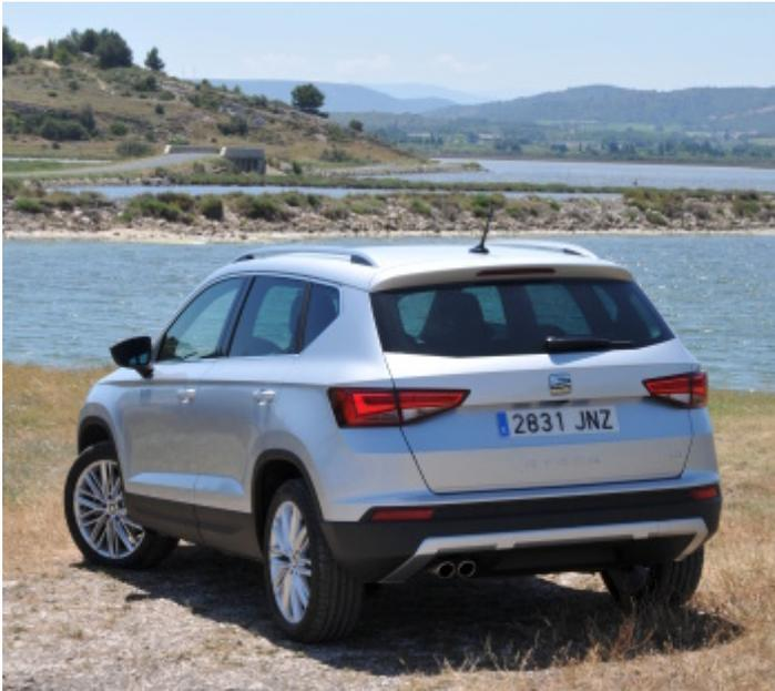
The test drive took the Ateca from the Seat factory in Spain all the way to the North of Europe. Despite driving at high speeds for extended periods of time, the Ateca used just 6 litres per 100 km (47 mpg). An economy run resulted in 5 litres per 100 km (56 mpg). This great mileage is also thanks to "cylinder on demand". When little power is required, two of the four cylinders do not receive any petrol, which saves fuel.
