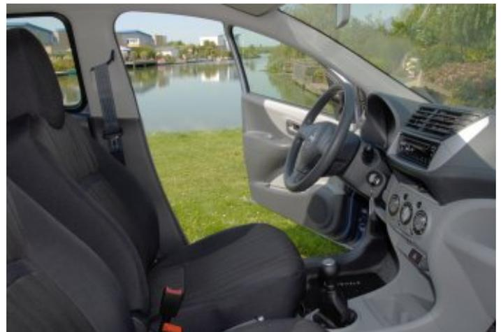
Oddly enough the integrated headrests are too low, so they do not contribute to safety. The mirrors are not adjustable enough for tall drivers, to provide a clear picture of what's happening behind the car.
