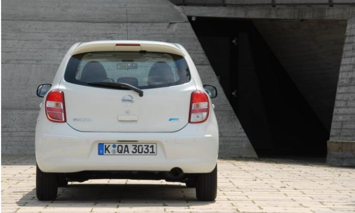
Nissan promises the car can do 4.1 litres per 100 km (110 mpg). So, after the fun and play, the speed was reduced to test the Micra's green credentials. On a route with city traffic, back roads and highways, the combined fuel consumption was a mere 4.7 litres per 100 km (97 mpg). That is much less than the basic Micra and even more frugal than many other compact cars.
