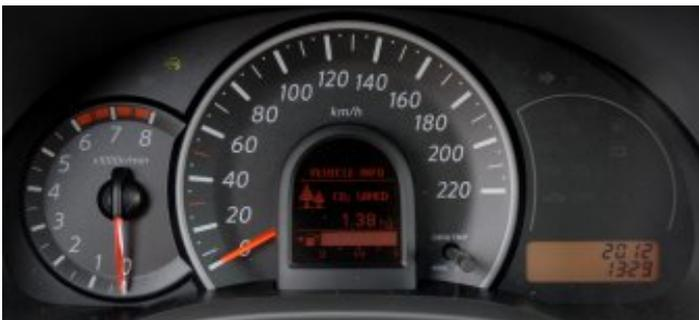
Of course, the Micra features a stop/start mechanism. This works so quickly that it is never disturbing to the driver. An interesting detail is the trip computer, which shows the amount of CO2 saved while the engine is stopped. When started again, the same display is used to show the actual and average fuel mileage. For some strange reason a shift indicator is lacking.
