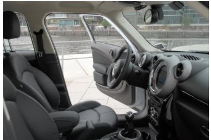
The test car is fitted with the optional satnav. Its display is placed inside the huge, central speedometer. The combined audio, communication and navigation system is controlled by a single joystick and reminds of BMWs "iDrive".
