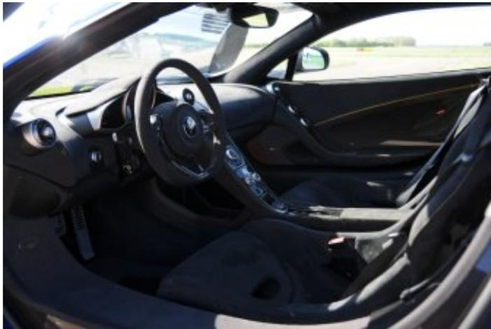
The seats are always tailor-made. The mechanics required for adjustable seats are just too heavy. Oddly enough, the steering wheel is (electrically) adjustable.
