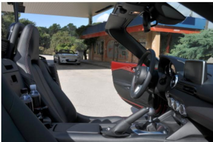
The passenger has an extra problem. The catalytic converter is mounted in the centre console. It takes up valuable legroom and the heat from the catalytic converter can be felt around the knees.
