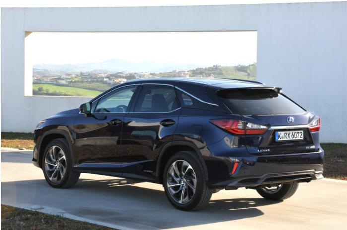
This choice benefits a car like the RX in several ways. The most important is that this traditional form of hybrid drive is more effective on long distances. Also, the RX450h doesn't have to be plugged in. Finally, because less batteries are required, the car is lighter and that benefits handling.
