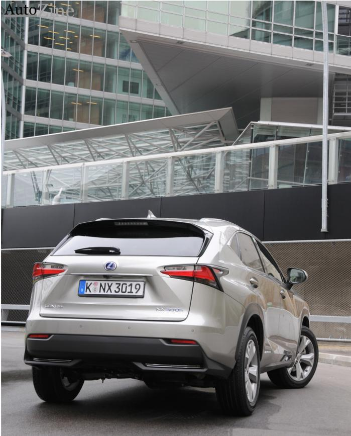
The computer decides which engine is used and when energy is being recuperated. The driver can influence this by choosing either the "eco" mode (which aims at maximum efficiency) or "sports" mode (which uses both engines at the same time for maximum performance). In city traffic, the NX can be powered by the electric motor alone but only for about 3 kilometres.
