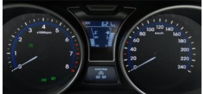
Because the Veloster draws so much attention to itself, the test drive was done at a higher speed than usual. Despite this, average fuel consumption was 71.8 mpg (factory figure: 81.3 mpg).
