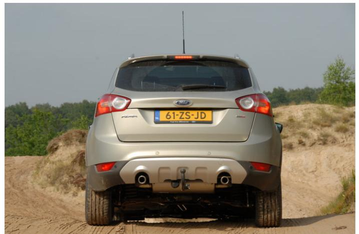
The under body protection is continued all the way to the bumpers, which gives the impression that the Kuga is very capable. Because the wheels are located on the extreme corners, the overhang is minimal and in theory the Kuga should be able to climb very steep ascents.
