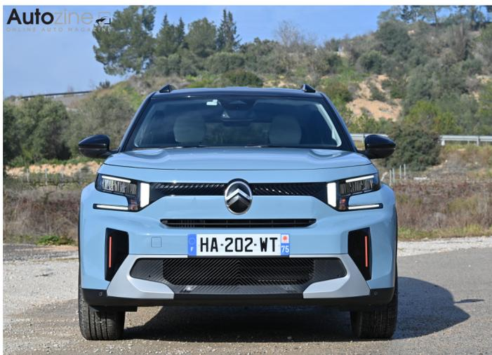
The angular design serves more than looks and a low price (flat/angled panels are easier to produce than round/wavy shapes). In fact, the C3 AirCross is available as a seven-seater. To make room for a third row of seats, the AirCross is longer, wider and taller
