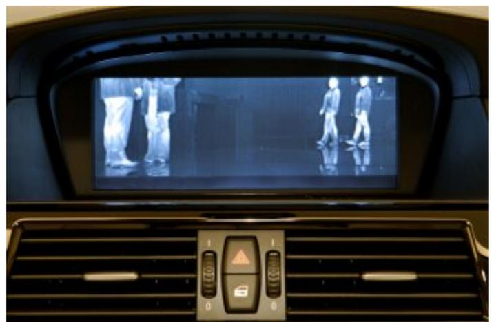
The first of these is the Night Vision system which displays pictures from a thermal imaging camera on the central screen which is located on the dashboard. A short nocturnal test identifies that this system is best utilized as an interior mirror: the driver can keep his eyes on the road, but an occasional glance of the screen gives a more comprehensive view of the driver's surroundings. Night Vision helps to identify those dark details which the naked eye might miss.
