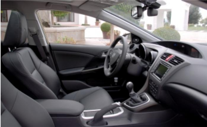
What's left is an unusual use of space. The fuel tank is placed under the front seats, meaning they cannot be adjusted in height quite as much as one would prefer. Despite the coupé-like layout, the driver isn't submerged in the many displays but instead looks down on them. Head and legroom in the front are fine, yet it does take some time to find an ideal driving position.
