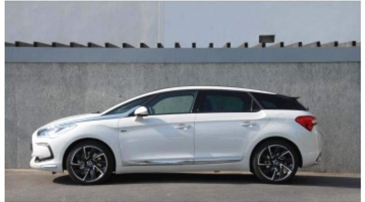
As an extra added bonus, Citroën's "Hybrid4" technology offers four-wheel drive. Although ground clearance isn't sufficient for off-road driving, crossing a patch of loose sand proved to be no problem. By engaging "Zev" mode the driver requests the system to run on the electric motor only, whenever possible. This is possible for 3 km at a maximum speed of 70 km/h.
