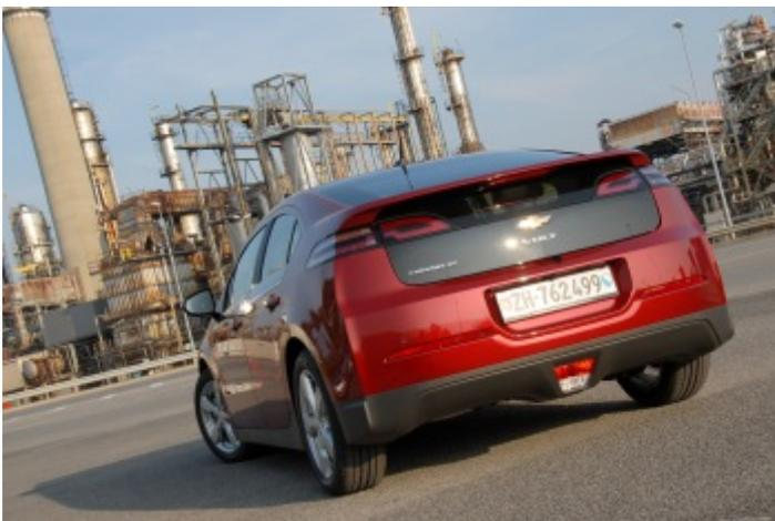
During the first test drive 121 km was covered; the first 80 km using the electric engine and after that 41 km using the "range extender". The average fuel consumption over the test whole drive was 5.13 litres of petrol plus 10.5 kW-h on electricity. The combined energy consumption was 4.2 litres per 100 km (67 mpg).
