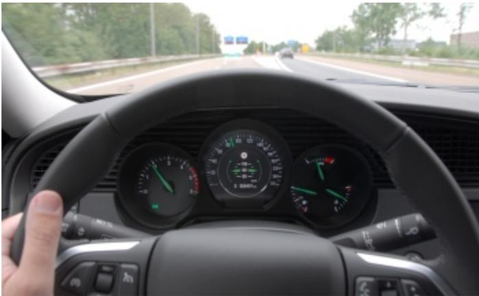
Also very nice to look at is the "head-up display": essential information like the actual speed and instructions from the satnav are projected against the windscreen. In this way the data seems to hover in the landscape, right in view of the driver. A display between the traditional speedometer and rev counter shows additional information like the average fuel consumption. In the same display a camera reads traffic signs and shows data, like the actual speed limit as a reminder.
