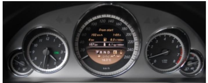
The remaining amount of gas can be read on a display between the speedometer and rev counter. Changing from one fuel to the other can be done via the computer.
