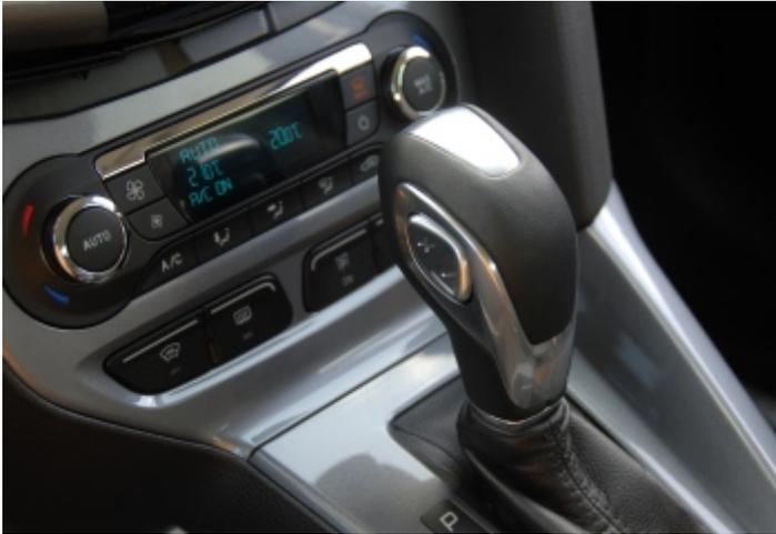
Regrettably the "Powershift" gearbox isn't in tune with the driver and always shifts too early or too late. The solution is for the driver to shift sequentially, but that can only be done by a cumbersome switch on the side of the gear lever.
