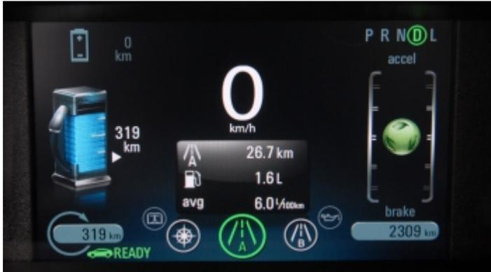
Its true fuel economy depends on the ratio between the distance travelled on the electric motor and the petrol engine. During the official "European test cycle" Vauxhall measured a fuel economy of 183 mpg.
