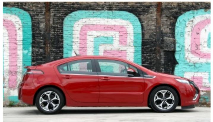
To see what the Ampera was capable of, motoring journalists competed in an eco run. They drove between 39 and 72 kilometres (24 and 44 miles) on the batteries alone. Once the batteries are depleted, the petrol engine starts automatically. This can be heard and felt, but isn't disturbing.
