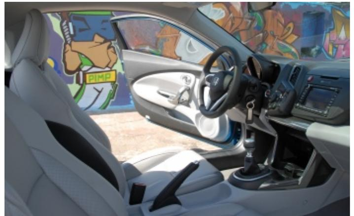
Just like most other coupés the CR-Z is hard to look out of. Vision in the rear view mirror is obstructed by the split tailgate. To optimise aerodynamics the outside mirrors are very small, which also doesn't improve visibility.
