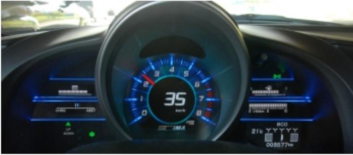
Behind the steering wheel deep, round dials can be found, just like in a classic sports car. However, the lighting seems to be inspired by a UFO. When the engine is ignited a blue glow illuminates the dials. Depending on the driving style, the colour changes ("Ambient meter"). When driving fast, the ring around the rev counter is red; driving efficiently results in a green light.
