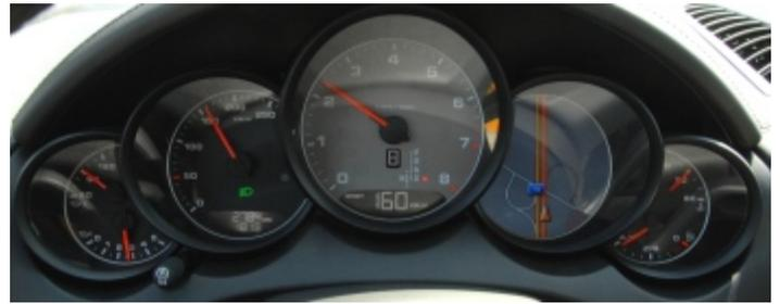
The dials have been copied verbatim from the Porsche 911. A large rev counter takes centre stage. Next to the very small speedometer there's a more accurate, digital speedometer. A real work of art is the round (!) display for the sat nav, to the right of the rev counter. This isn't just pretty to look at, but also more easy to read than a traditional display in the centre console.
