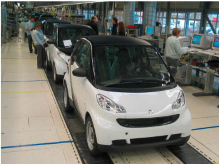
The last step in the process is quality control. On a rolling road the engine and brakes are tested. In a wet cell the cars are checked for watertightness; this goes for all cars, not just the convertibles. Finally a visual check is carried out. If any problems are found, the car is separated and fixed by a specialist.
