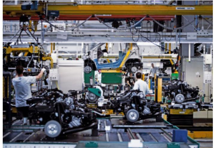
Although the car doesn't have any body panels yet, the Brabus versions can now be recognised by the double exhaust pipes. The tyres, including the rims, are delivered in piles of four. Again the Brabus stands out because of its unusually wide tyres. The use of robots in Smartville is minimal; building a Smart ForTwo is mostly done by people assisted by custom-made tools that make the process run smoothly and efficiently.
