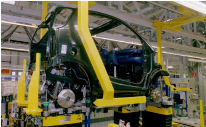
After the safety cell is protected by a coating of (powder) paint, the dashboard is installed. This is supplied by Continental, which is best known for its tyres. Now it becomes obvious how complicated building a car actually is. Just the interior can be executed in 5,000 different ways because of options and colour schemes. On the work floor merging the chassis and the dashboard is called the "engagement".
