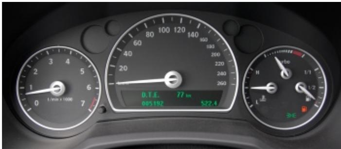
Another well-known Saab invention is the "Nightpanel". When driving in the dark all lighting in the dashboard can be switched off, except the speedometer. This makes driving in the dark much more pleasant to the eyes.
