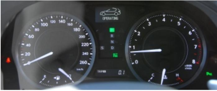
The (aluminium) roof opens and closes in 20 seconds. The process speeds up and slows down right before finishing, just because it feels better that way. The parking sensors in the rear bumper are also used to check if there's enough space behind the vehicle to open the boot. The whole process of opening and closing the roof is also visible on a little display between the speedometer and revcounter.
