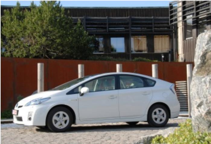
The fact that the Prius III is fitted with a stronger petrol engine (98 bhp / 142 Nm) than its predecessor, is most evident in the "power" mode. In this mode the Prius instantly reacts to the slightest movement of the throttle and performs very well.
