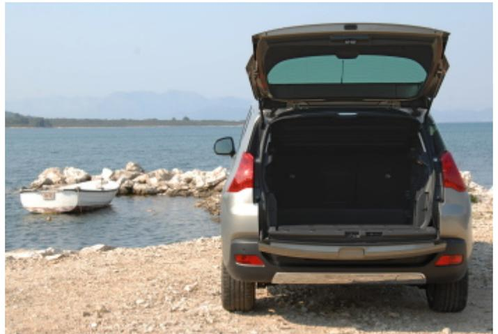
The boot is accessible via a split tailgate. To load small luggage it's sufficient to open just the top half, which takes less effort. The bottom part of the boot lid pivots down, so one can also sit on it.
