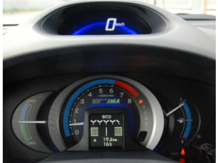
Most educational is a graph bar that grows in one direction when accelerating too fast and to the other side when braking too hard. The latter may seem illogical: but braking hard is a sign that the driver didn't anticipate traffic properly. Also the batteries have more time to charge when braking carefully. In short: the smoother the driving style, the more economic.
