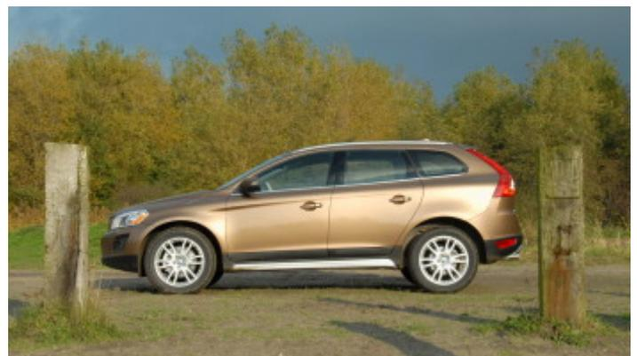
The test car is fitted with a D5 diesel engine; the strongest one on the price list. This remarkably silent five cylinder delivers 184 hp / 400 Nm. Even at low revs the power unit is very strong, but it's never frisky or eager. Only at full throttle this most powerful XC60 is willing to perform.
