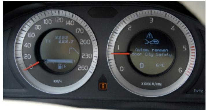
"City Safety" only works when the driver doesn't actively participate. In other words: the speed should be constant. After braking automatically, the car will be stopped for one full second. After that the computer releases the brakes. Those who didn't recover from the initial scare, will hit the car in front after all. Finally, the laser only works on reflective surfaces; therefore the XC60 doesn't brake for bicycles or pedestrians.
