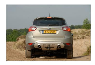
The under body protection is continued all the way to the bumpers, which gives the impression that the Kuga is very capable. Because the wheels are located on the extreme corners, the overhang is minimal and in theory the Kuga should be able to climb very steep ascents.
