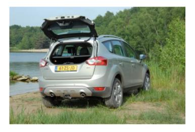
According to the latest trend the tail gate of the Kuga can be opened in two separate parts. For big loads the whole rear door has to be opened. To allow for smaller luggage only the top half can be opened. However, this upper half is made so heavy that it takes almost as much force to open the whole boot lid. This defeats the purpose of having a split tail gate.
