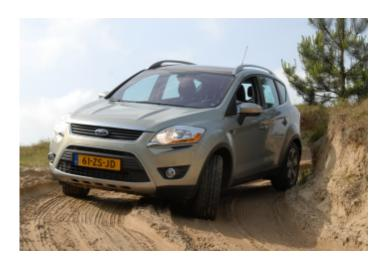
The (optional) automatic four wheel drive system is very effective. Normally the Kuga uses front wheel drive, but when needed the rear wheels will automatically assist. Thanks to this system the Kuga could even prove its talents off road.
