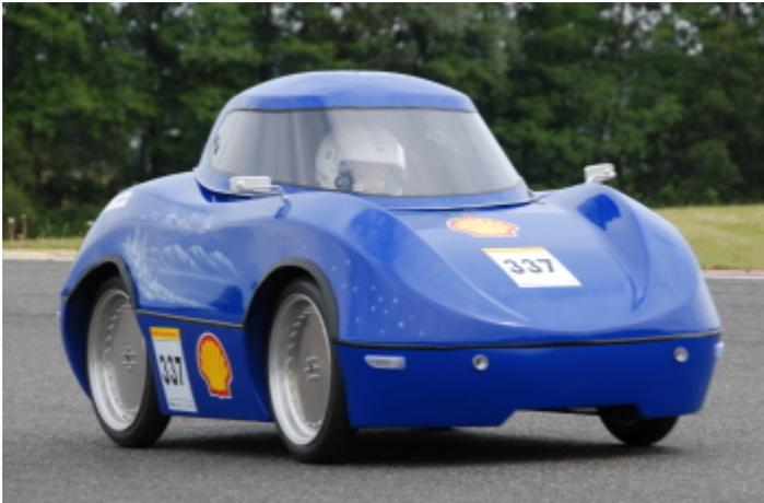
One of the best looking cars comes from Denmark. The "Roadrunner" resembles a miniature Jaguar, but runs on a newly developed fuel. According to the team "Dimethyl Ether" offers all of the qualities of diesel, but can be made from bio-mass. The result: 265 km on 1 liter.
