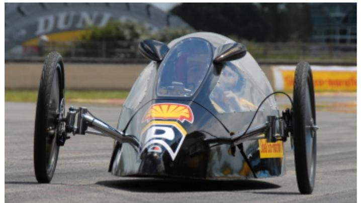
The "Prototypes" resemble "cigars on wheels", where the drivers lay down instead of sit down. "Gas guzzling" things like a roof and doors are no longer required. The technical specifications are much more extreme, the fuel economy sensational: 3,000 km out of one liter of fuel is no exception.
