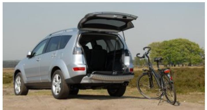
The two-part tailgate is extremely handy, making loading and unloading so easy. The lower section of the tailgate can double up as a seat for a maximum weight of 200 kilograms. Unfortunately the upper section does not open high enough, potentially risky for taller people.
