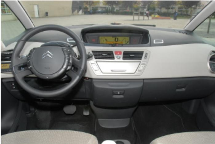
With paddles behind the steering wheel, it is possible to choose the previous or next gear. Unfortunately the paddles don't turn with the steering wheel, which was a poor decision on Citroen's part. This system which originated from the sports model was designed to allow gear changes whilst moving through turns. The hands would remain safely on the steering wheel.
