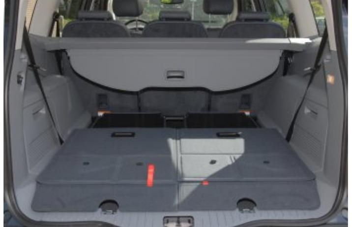
The "Ford Fold Flat System" makes it really easy to fold down the seats to make the luggage space even larger. The seats don't need to be expanded but with two easy movements can be laid flat. A massive flat and easily accessible loading floor is the result. For those that do not choose the second rear seat can have a moveable loading floor which makes loading and unloading more simple.
