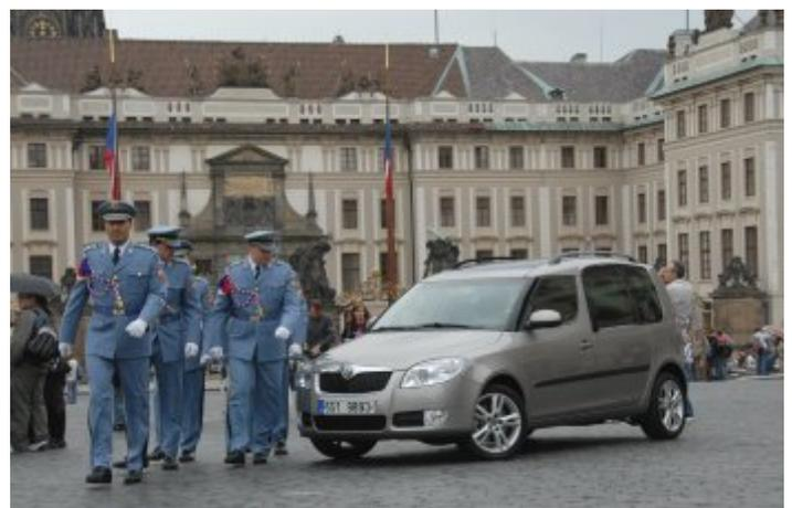
The front half of the Roomster is a normal car, the back half is an MPV. In this simply way Skoda solves a couple of complex problems. A traditional monospace, also known as MPV (multi purpose vehicle) is in essence no more than a van that evolved into a roomy family car. No matter how refined a modern MPV is, the ride quality is still affected by the poor road holding (high centre of gravity) and high gasmileage
