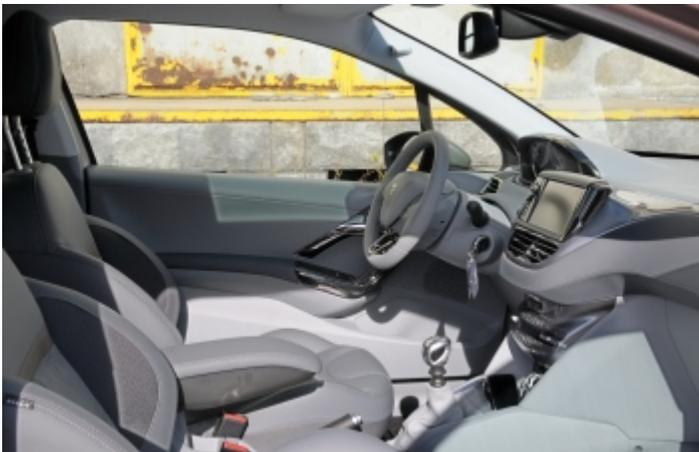
In most cars the dials are placed directly behind the steering wheel; the driver looks through the steering wheel to read the speedometer. In the 208, the dials are placed more towards the windscreen so the driver looks at them over the steering wheel. This makes them easier to read and mimics the effect of "head up display" (projecting information on the windscreen).
