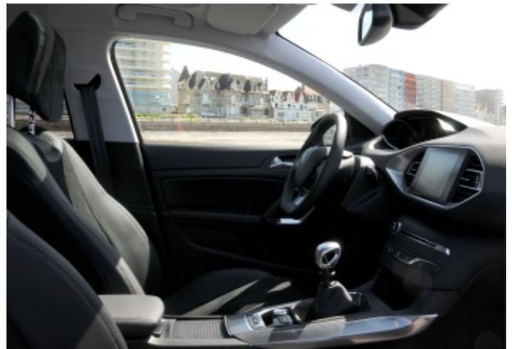
Another thing that makes the 308 special is the minimum number of buttons and dials on the dashboard. Almost all functions are controlled via the centrally located touch screen. This even goes for the climate control. What remains are a single volume knob for the stereo, a button for the hazard lights and the controls of the air vents.
