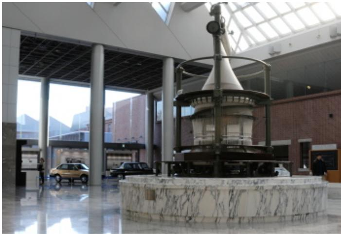
Do take a look at the circular loom in the central hall. With a traditional loom the spindle has to go back and forth and that means one empty and thus unproductive move. The circular loom makes a constant move, meaning no time is wasted. This is the very first sign of the unique way of approaching business that is now know as "The Toyota Way".
