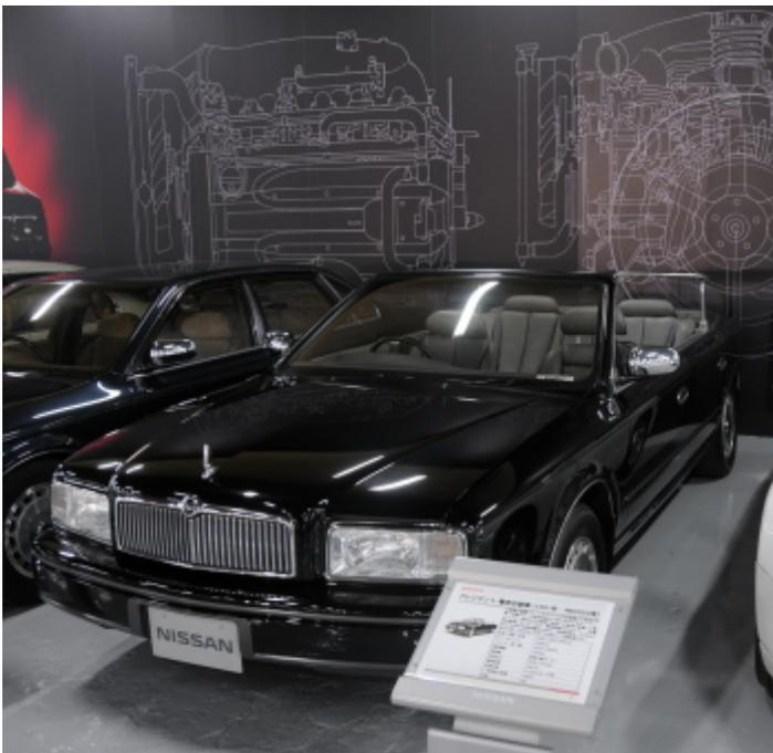
In 1991 Nissan was asked to build a bespoke car for the president. An existing model was converted into a cabriolet, with raised seats in the back. Since the car was to be used in enclosed spaces (like a stadium) an electric motor was installed.
