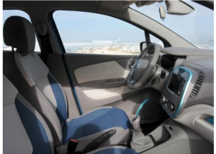
The cabin can be executed in a dark or light tint, after which many elements can once again be painted in contrasting colours. The seat covers are zipped in place, so they can be removed and washed. They can also be replaced, so the cabin will look like new even after many years of wear and tear.
