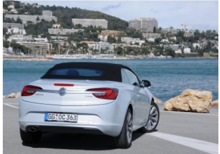
If desired, the roof can be opened or closed while driving at speeds of up to 30 mph. This takes 17 seconds. More important is the refinement of the mechanics responsible for operating the top. All electric motors, hinges and other parts operate very quietly.
