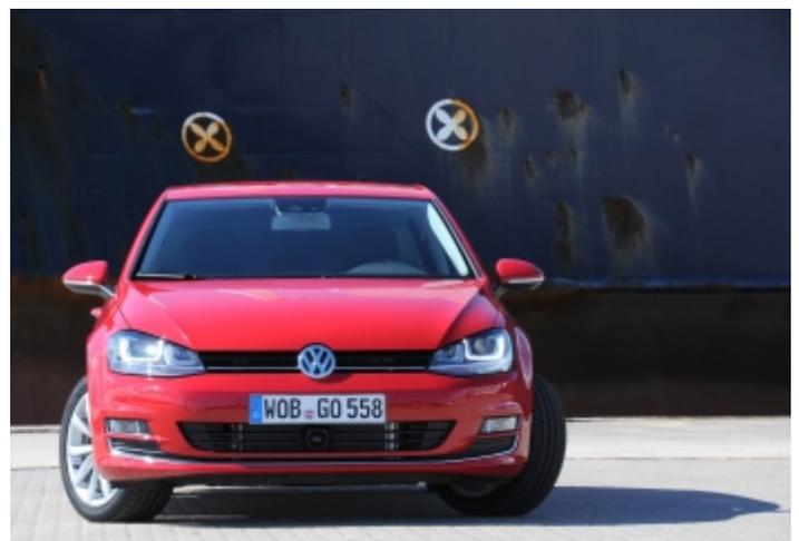
To offer more cabin space the Golf VII is longer. The wheelbase has increased by 26 mm and the front wheels have been moved forward. At the same time the car has been lowered to improve aerodynamics and improve fuel consumption. Recently Volkswagen gained a lot of experience with composite materials, which make a car both stronger (read: safer) and lighter. Compared to the previous Golf the new generation is about 100 kg lighter.
