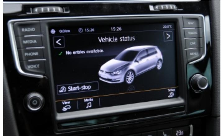
A large display dominates the dashboard, even on the base level of the Golf VII. The user interface resembles that of a mobile phone. Of course, the audio and communication system can be integrated with a phone or MP3 player. To make the screen easier to read VW implemented a "proximity sensor". This means that menus only appear just before the hand actually touches the screen.
